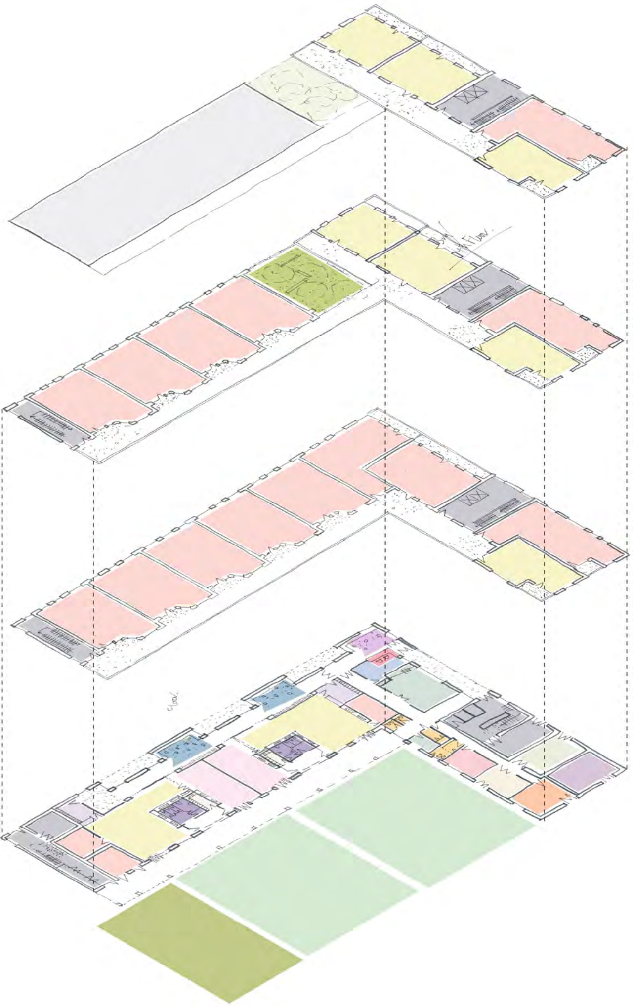
Exploded plan showing older person's housing above the nursery ground floor plan
